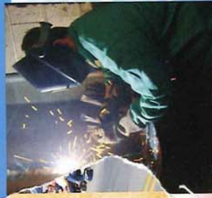
Anson Hatfield works at getting his vertical stick weld perfect.
